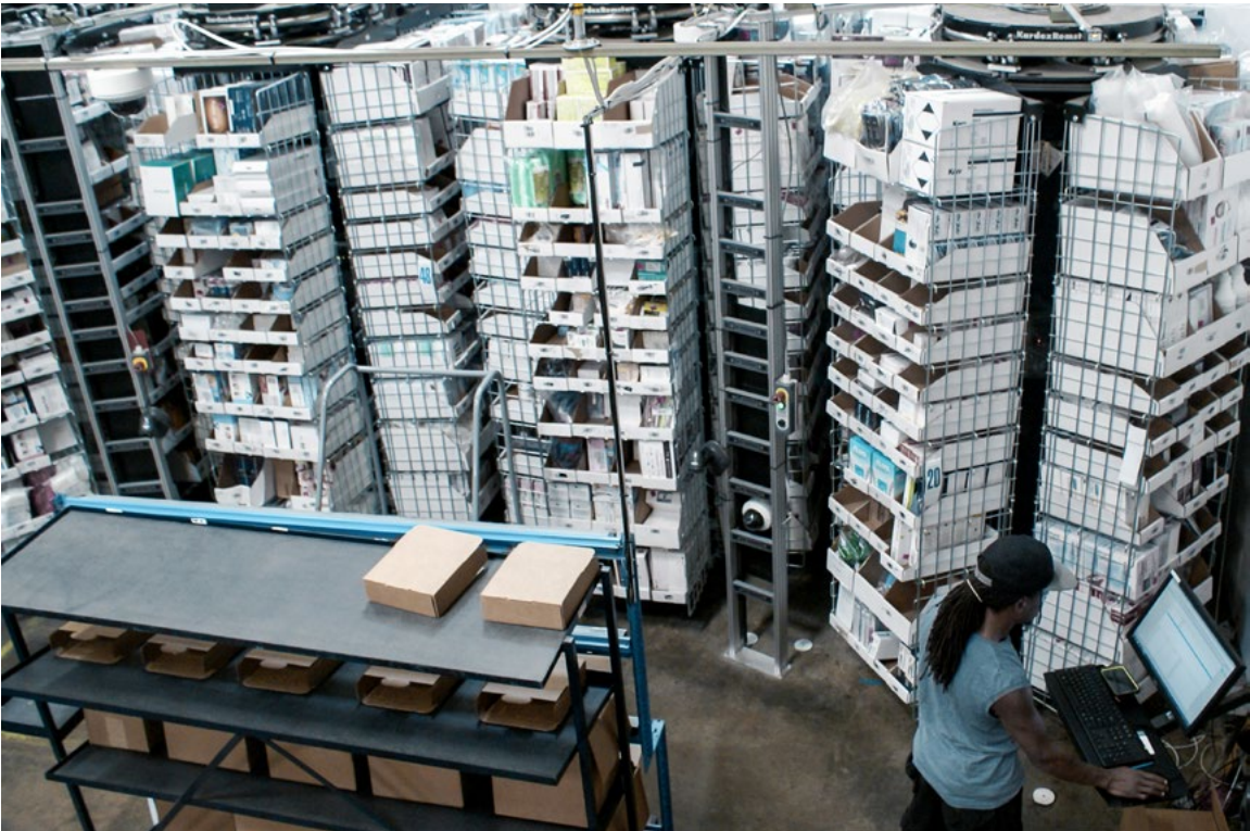
Horizontal Carousel Modules with Light Towers
